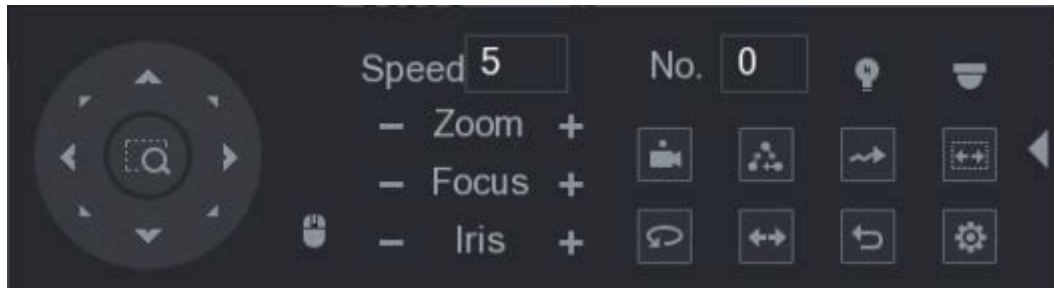
Figure 5-63 Expanded PTZ control panel
